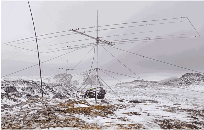
Figure 7 Moxon and Vertical Antennas (W7XU Photo)
