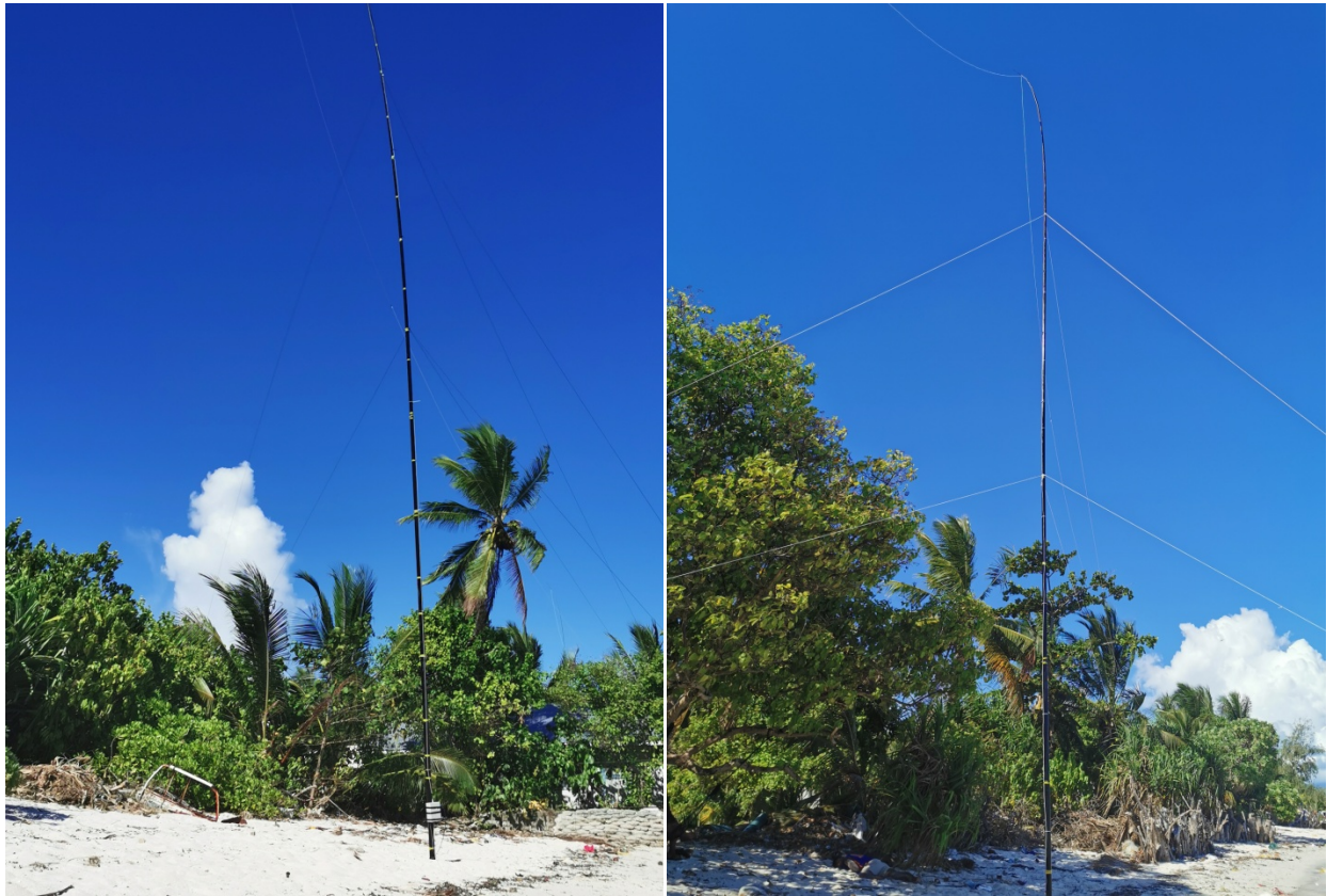
Our 2 Vertical antennas for low bands, both of them used on 160/80/40m bands
