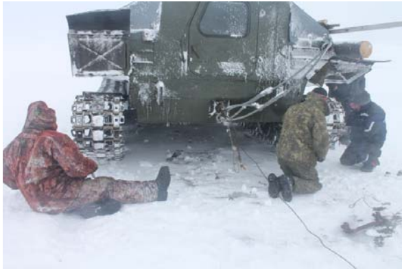
Fixing special hooks to tracks
