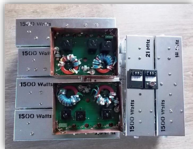
Perfo Box 1500 bandpass filters and Four-square relay switch units by RA6LBS (LBS)
