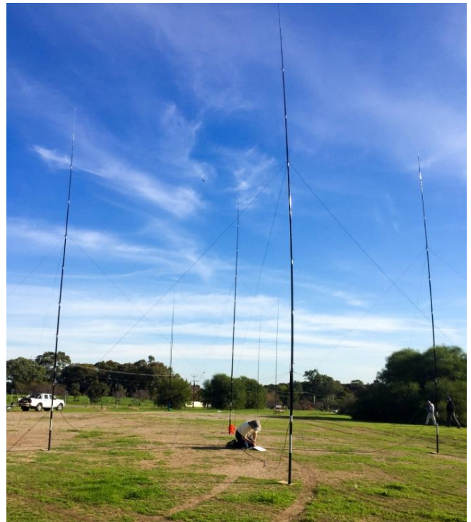
Photo 4 - Tune & Test Day in Adelaide 30 + 40m 4-square arrays
