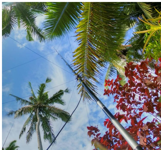
Photo 31 – 30m 4-square element on 10m
