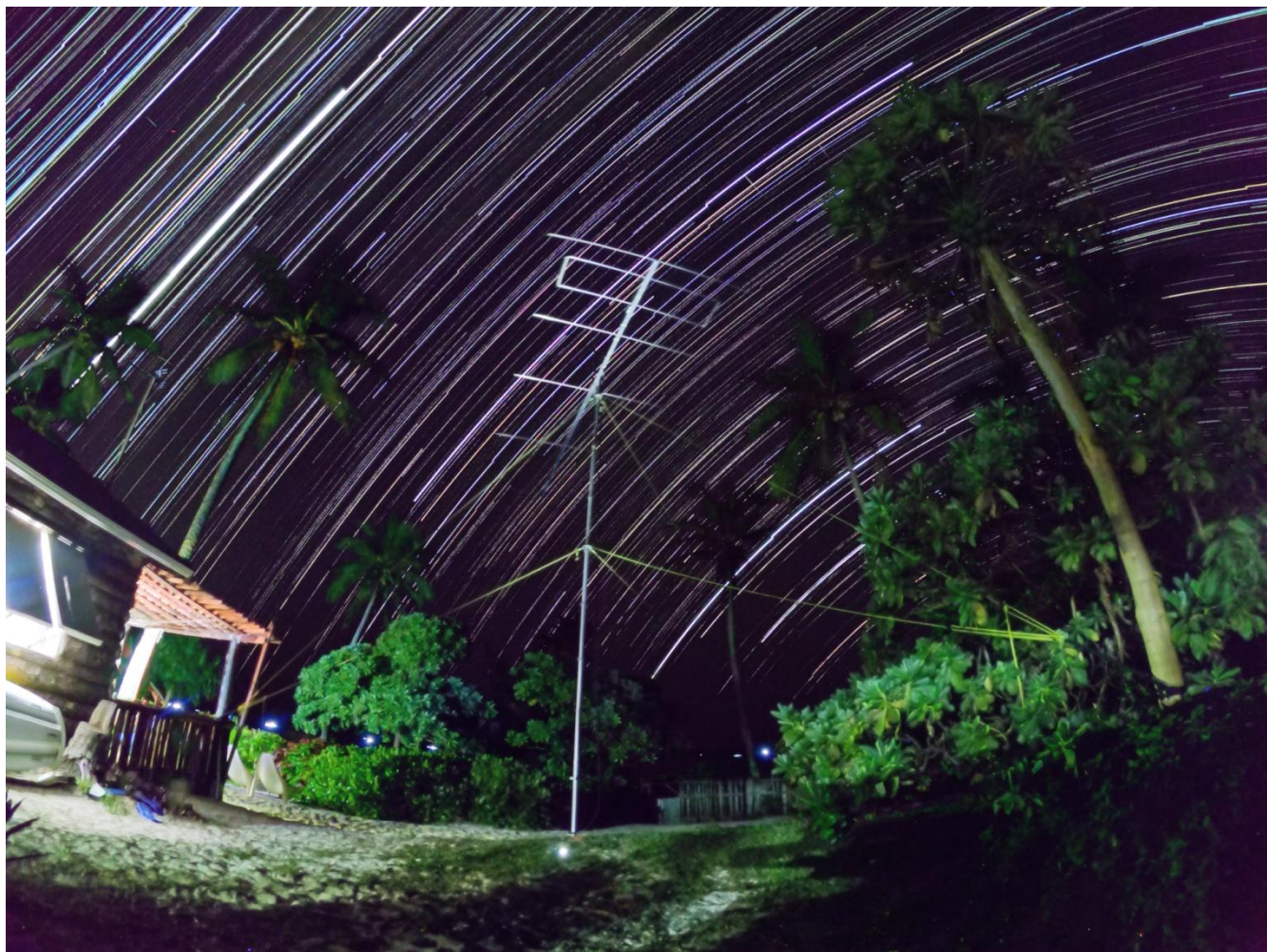
Photo 32 – 6m EME Array by Star Light
