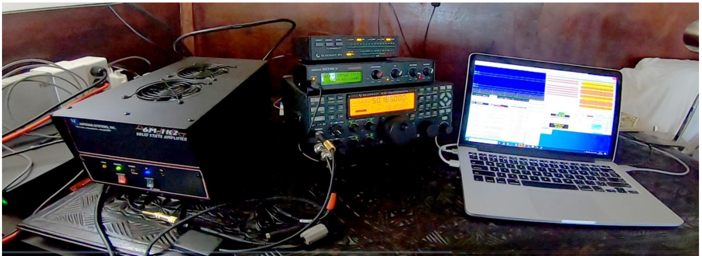
Photo 17 – 6m EME station – M2 Systems M6-1K2 Linear, Elecraft K3S, Elecraft W2 Watt Meter Eltek 2kW 50V Power Supply, Microham Keyer II and MacBook Pro
