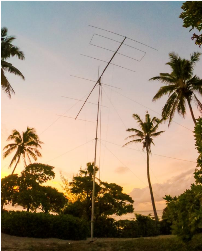
Photo 23 – 6m EME Yagi on its Spiderbeam™ Mast
