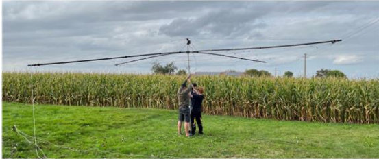
Testing the setup of a Spiderbeam for 10m, 15m and 20m in advance of 8R7X.
