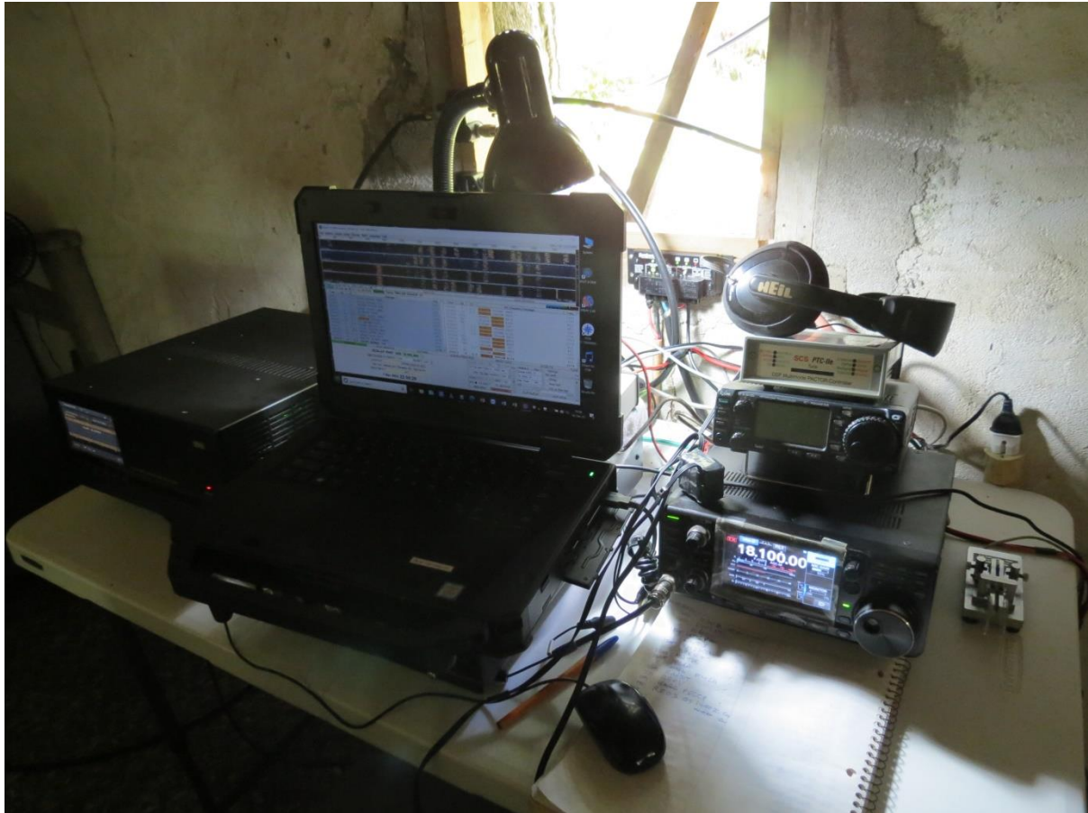
The operating station, with the ACOM 600S linear, IC-7300 and IC-706 radios, and PACTOR modem
