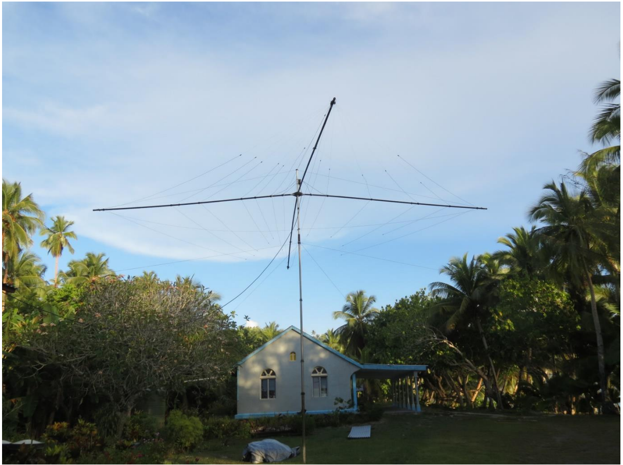
The fully-assembled and mounted Spiderbeam antenna
